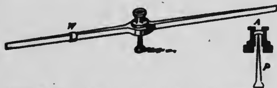
FIG. 139. — A magnetic needle, with a cross-section to show the mode of hanging. P , pivot; A , cap of agate with hollow beneath to rest on the pivot; W , adjustable weight to counteract the dipping tendency.
